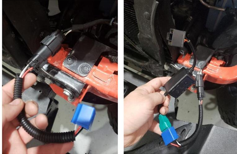
4. Once all necessary connections have been made you may mount new adapter rings using factory bolts.
