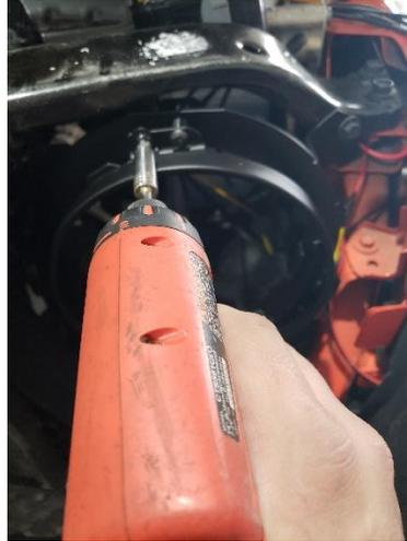
6. Plug in new headlight assembly and align the notches on assembly with new adapter bracket and screw in the ring to hold new assembly in place.
