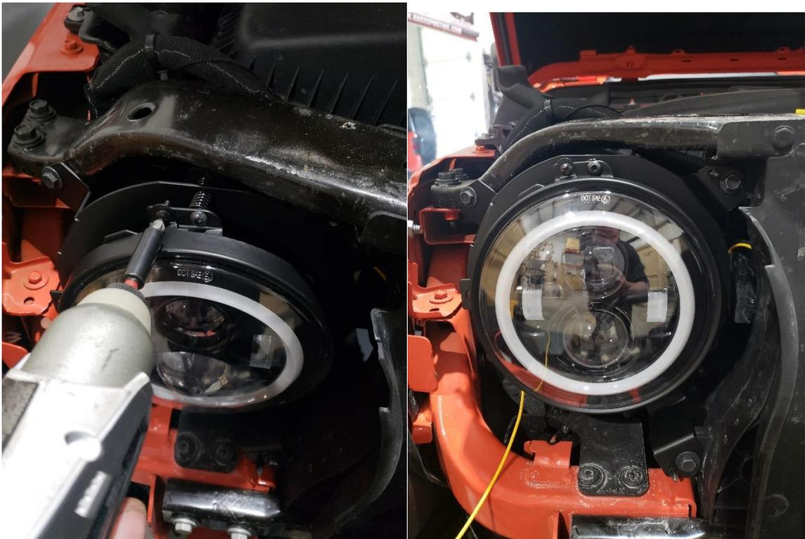
**Test the new lights and make sure everything is functional, you may also check headlight adjustment if it off the you may adjust the headlights using the adjustment screw.**
