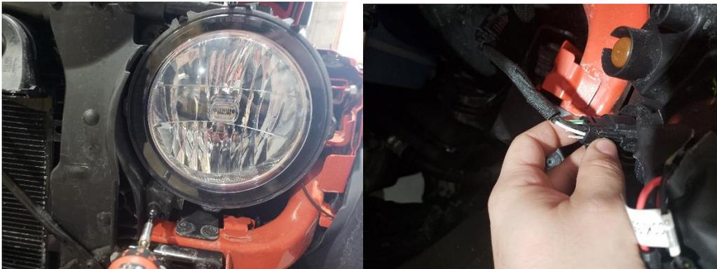
3. Once the assembly has been removed, you may plug in your adapters. One adapter is to convert the plug over to an H4 plug, the next plug is to interface the new 7" round to the vehicle.
