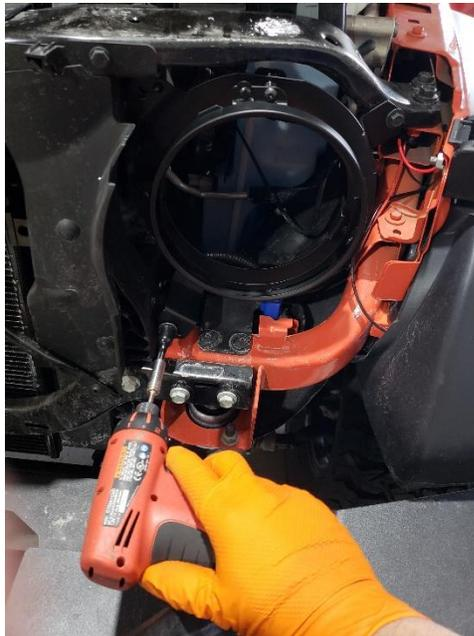
5. Next step is to remove the outer ring by removing 3 phillips screws.
