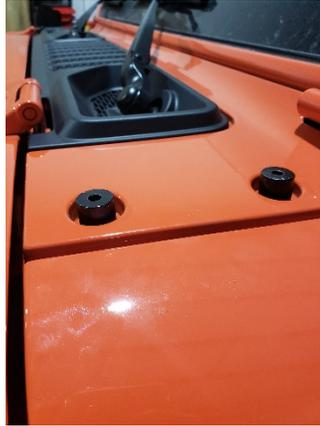
3. Once the brackets are mounted on the hood you may mount light bar to the hood brackets. Run the wire through the crevasse between the fender and wiper cowl of the vehicle.
