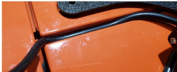
4. Start running relay harness to the battery and switch to desired location in the inside of the vehicle.
