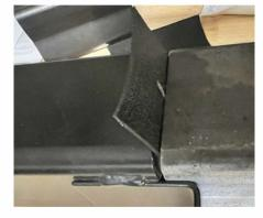
3) With the Rubber Shim on top, reinsert the Hitch Bar into the hitch. Ensure that the rubber slides into the Hitch along with the Hitch Bar.
